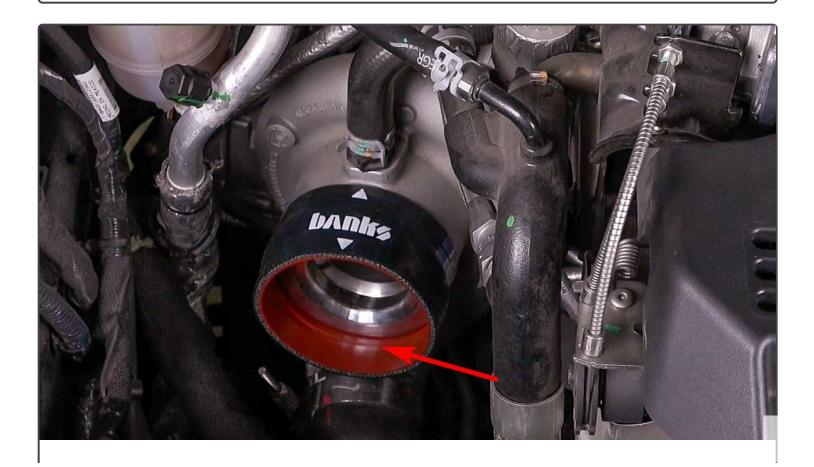
Slip the Banks hose onto the turbo with the arrow aligned to the breather hose on the turbo.
