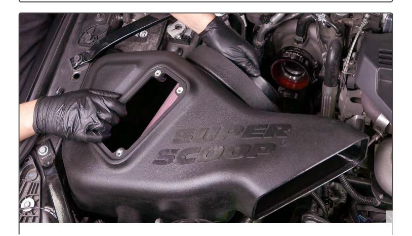
Insert filter into the Banks housing and place the large hose clamp over the filter cuff.
