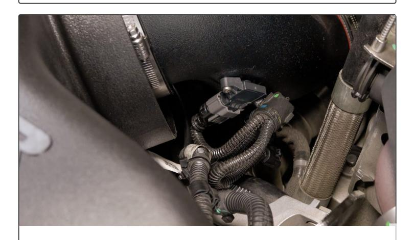
Make sure the sensor harness is tucked against the intake housing and away from moving parts.
